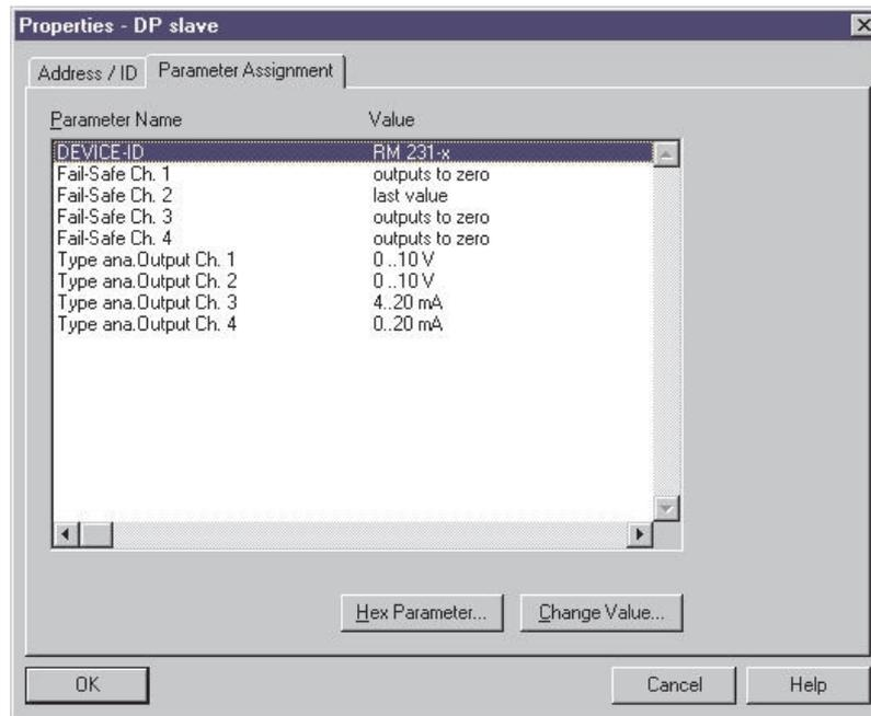
Example STEP7: Parameter of analog output module RM 231-x
