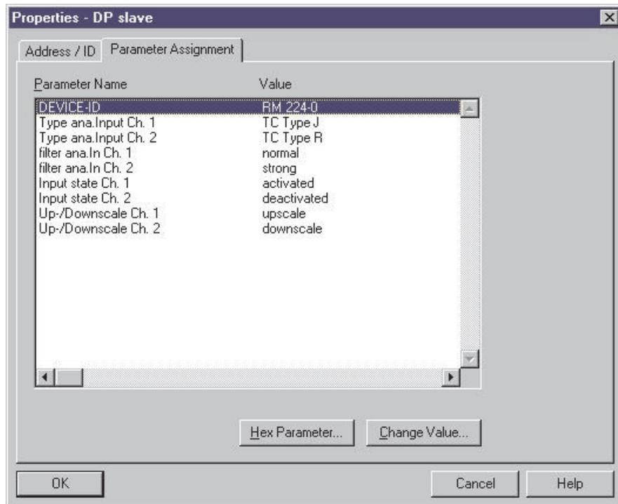
*Example STEP7: Parameter of thermocouple module RM 224-0*
