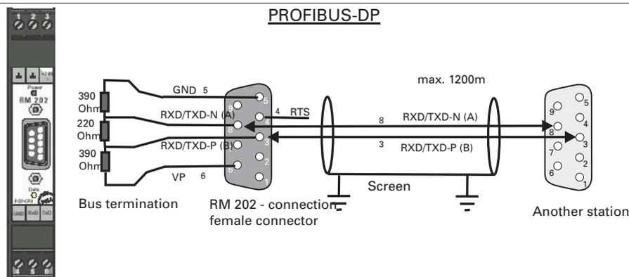
The construction of suitable cabling must be provided by the user, whereby the general cable specifications according to EN 50170 vol. 2 must be taken into account.
