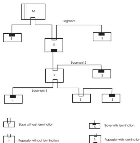
PROFIBUS systems are build as line structure. A PROFIBUS project can be extended by of connection of repeaters,
