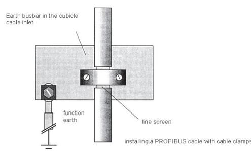
The bus is to be installed always with a minimum distance of 20 cm to other lines, which carry a voltage higher than 60 V. The bus cable is also to lay separated from telephone lines and cables, which lead into explosion protected areas. In such cases it is recommended to use a separate tin duct for the bus cable.
