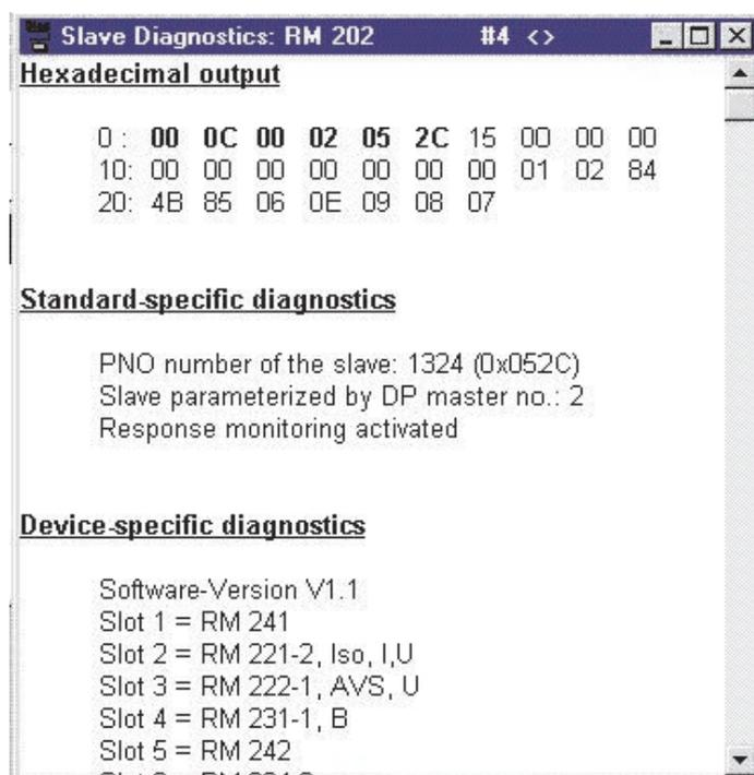
The following figure below shows the diagnosis of a PROFIBUS-DP slaves with activated 'extended diagnosis' and an error at the input 2 of the module in slot 8. As shown in the diagnostic message, a 4-channel temperature modul RM 224-1 is placed in slot 8. The error could be e.g. a sensor break at channel 2 of the RM 224-1 module.
