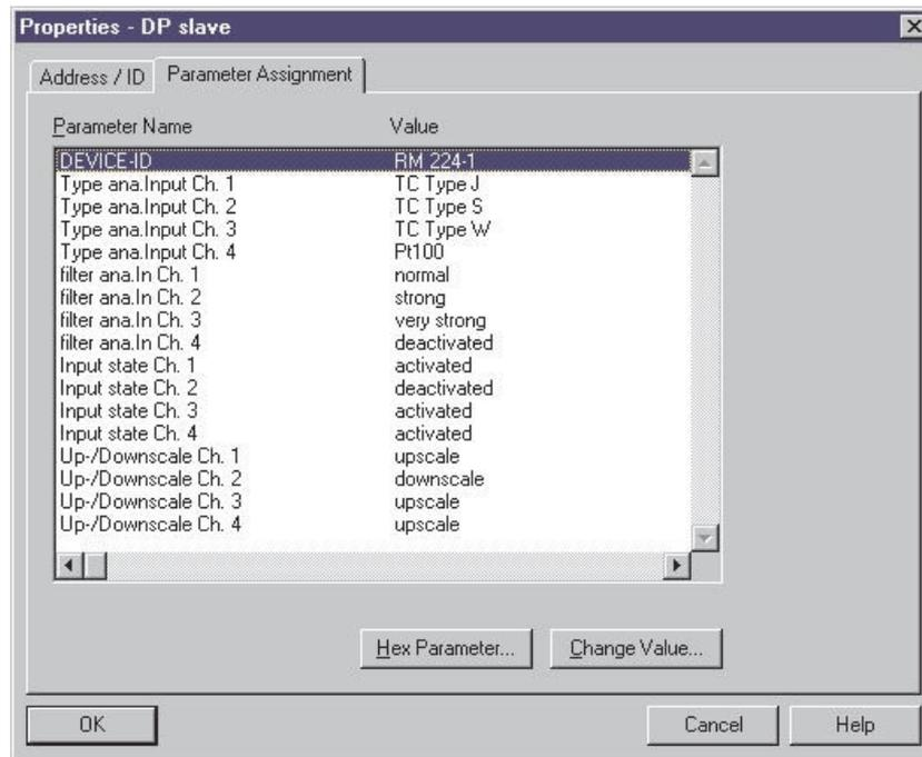
*Example STEP7: Parameter of temperature module RM 224-1*
