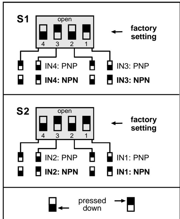
The **NPN-input** is suitable for direct connection of switches with NPN-output. The collector is be connected with the respective transducer supply, the emitter with the respective input (**factory setting**)
