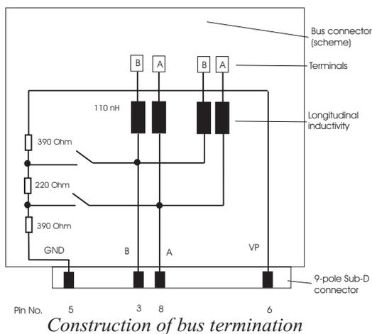
Bus terminal resistors adapt the impedance of the bus to the apparent impedance of the bus users. The input circuit of the attached field devices is substantially high impedance as the bus termination. By the termination of the bus cable at both ends of a segment with the termination resistors, it is guaranteed that
