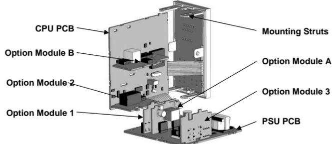
To access modules 1, A or B, first detach the PSU and CPU boards from the front by lifting first the upper, and then lower mounting struts. Gently separate the boards.
