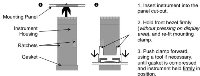
**CAUTION:** For an effective IP66 & NEMA 4X seal against dust and moisture, ensure gasket is well compressed against the panel, with the 4 tongues located in the same ratchet slot.
