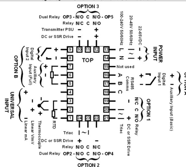
**\*Note:** This controller uses 3-Point Stepping Control. This requires two identical outputs (2 Relays, 2 Triacs, 2 SSR Drivers or 1 Dual Relay) for the valve Open & Close functions. See Output Usage 1-5 in Configuration Mode. At first power-up the message `GoTo Conf` is displayed, as described in section 7 of this manual. Access to other menus is denied until Configuration Mode is completed.
