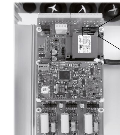
To change auxiliary supply voltage sold the correct link-jumper on Relay C board.
