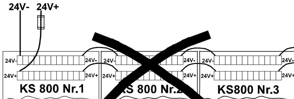
Faulty supply voltage connection with several KS800 units
